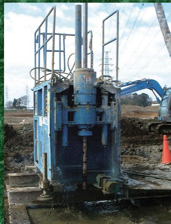
**Twin High-Pressure Cement Slurry Jets Rapidly Creates Improved Body with Large Diameter**
